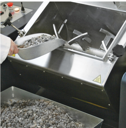
Asphalt mixer: aggregate loading operation
